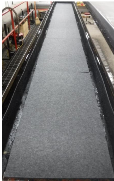
Photo No. 2 Unexposed Surface of the Test Specimen (Pre-test)
