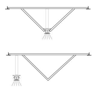
We realize that sprinklers are a necessary evil and part of almost every ceiling. Above are two suggestions for sprinklers when code requires that they drop to the lowest part of the tiles.
